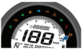
The TVS RONIN does an automatic self check every time whenever the ignition lock of the bike is turned 'ON'. The ABS warning lamp provided on the instrument cluster blinks and informs you that the ABS is under check.
