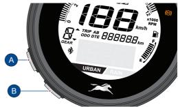
The 'Mode' (A) and 'Set' (B) buttons are provided to change between various modes and to set the some of the digital display functions of the instrument cluster. The sequence of modes and their selections are explained in detail below.
