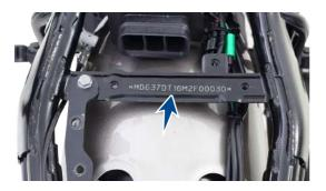
Frame serial number is engraved on the frame bellow the seat assembly as shown.
