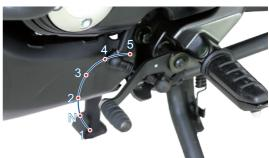
Lifting the lever up repeatedly engages all the gears in succession up to the fifth gear.
