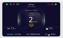
During forward movement the speed is limited to 10 km/h and during reverse speed is limited to 3 km/h
