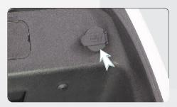
Your TVS iQube Electric S is provided with a socket for charging your smart phone even while you are traveling and it is located in the utility box below the seat assembly. Refer <a href="page No. 22">page No. 22</a> for usage details.
