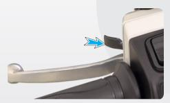
'Parking Brake' is another unique safety feature which protects your scooter from falling due to wheel rotation when it is parked with the side stand on a slope. Refer page No. 16 for details.
