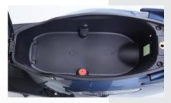
Utility box is located below the seat. Lift the seat by unlocking the seat lock as explained in the previous section, to access the utility box.
