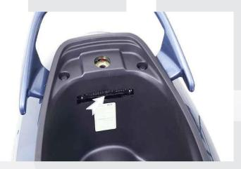
The frame serial number is stamped on the frame, at the rear end below the seat assembly. Open the seat assembly and remove the VIN cover to read the frame number.
