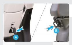
There are two bag hooks provided with your scooter to carry light luggage like carry bags weighing upto 3 kg. One hook is located below handle bar on the rear panel.
