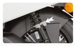
Your Scooter comes with Adjustable Shock Absorber, a first-in-the-industry feature. This allows you to adjust the required level of hardness / softness as per the usage requirement with just a push of a lever. Refer page No. 61 for details
