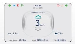
Press park assist switch once again, for shifting to reverse mode as shown, apply throttle to move.
