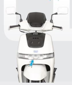
TVS iQube Electric S comes with a Automatic Headlamp ON (AHO) LED lamp which glows automatically once the ignition is turned 'ON'.
